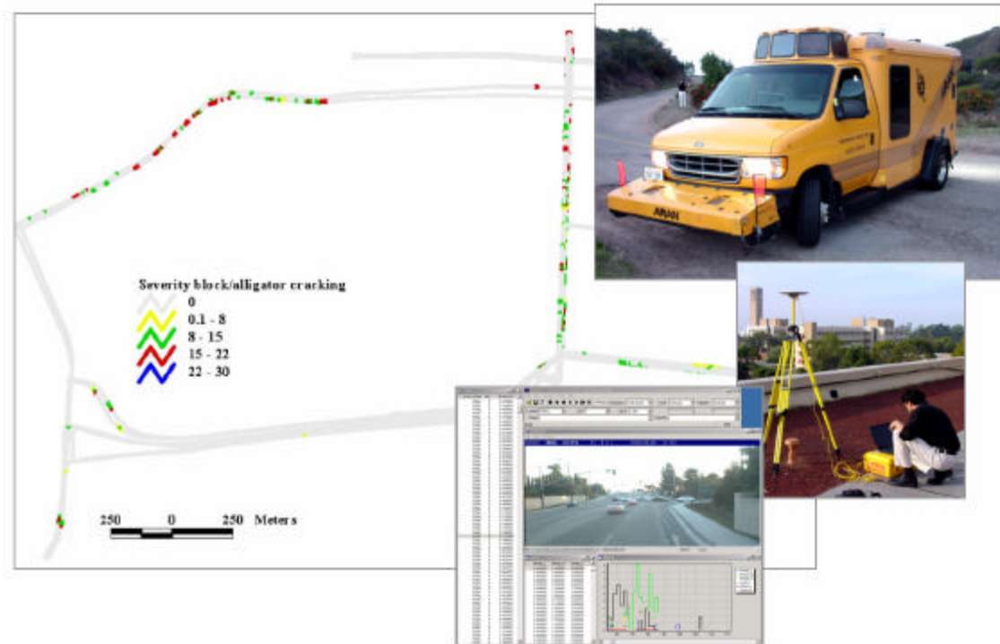
Figure 5: The Roadware pavement health survey with the ARAN survey vehicle, GPS base station, the video/road distress log and the resulting GIS database.
