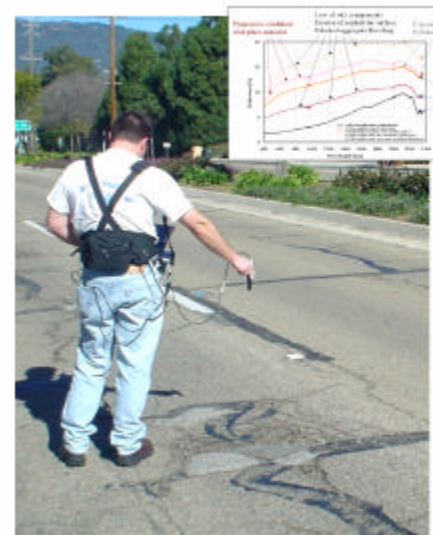
Figure 6: Acquisition of spectral samples of road surface distresses.
