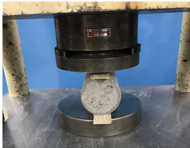
Figure 3.8 concrete split tensile strength test of cylinder
