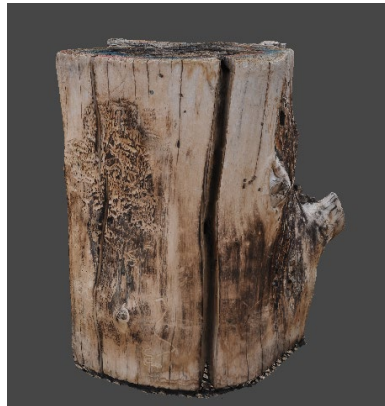
Figure 2.2 A planar image of the rendering of the result of photogrammetry imaging of 51 planar still photos of the cracked stump.
