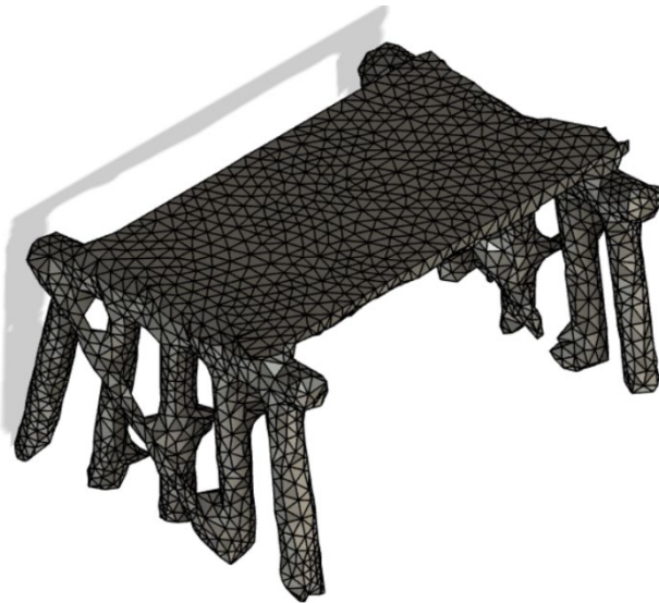
Figure 2.9 The final three-dimensional finite element mesh of the rail bridge following several intermediate steps moving from images to final numerical model.
