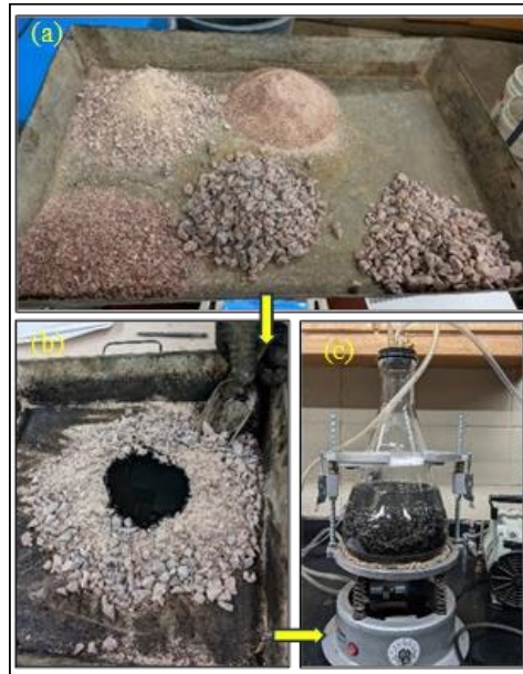
Figure 3.7 Photographic views of (a) batching, (b) mixing aggregates and asphalt binder, and (c) G_{\text{mm}} test
