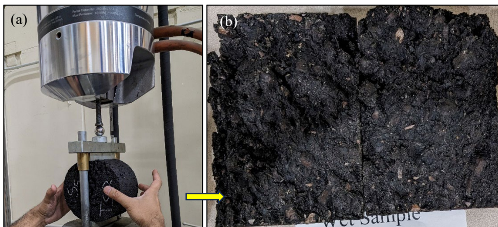
Figure 3.15 Photographic views of (a) TSR test setup and (b) failure surface
