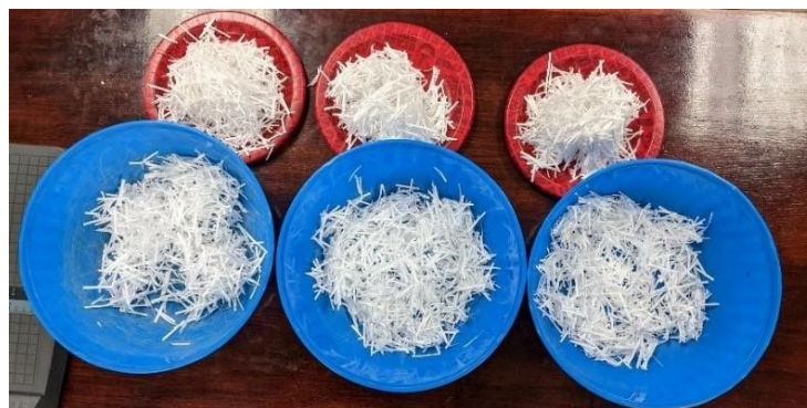
Figure 3.9 A photographic view of the EPM used for the preparation of asphalt mixes
