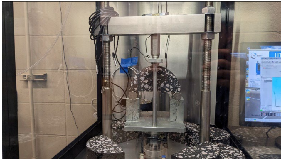
Figure 3.16 A photographic view of a SCB specimen subjected to loading in an AMPT
