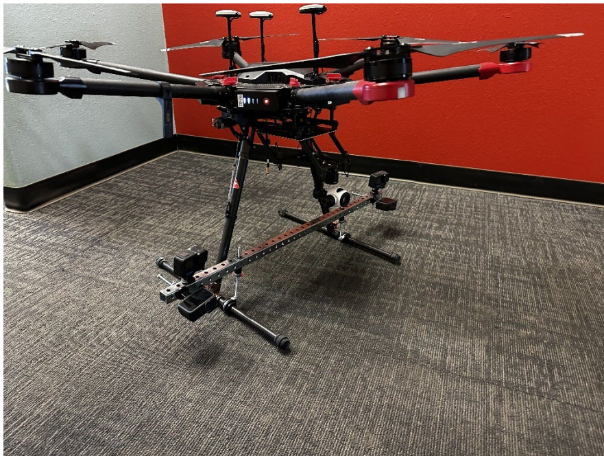
Figure 2.2 Dual stereovision camera rig attached to a DJI Matrice 600 Pro UAS: Matrice 600 Pro with attached camera rig
