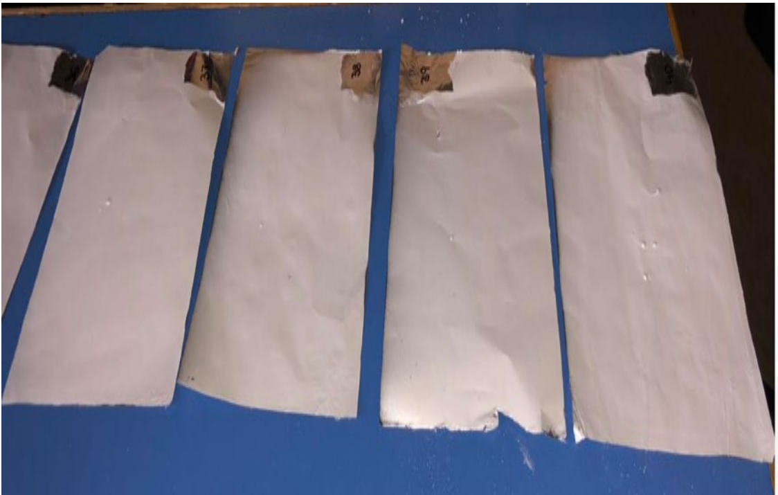
Figure 4.9 Photographic views of CNFs produced using solution 4 and static electrospinning technique
