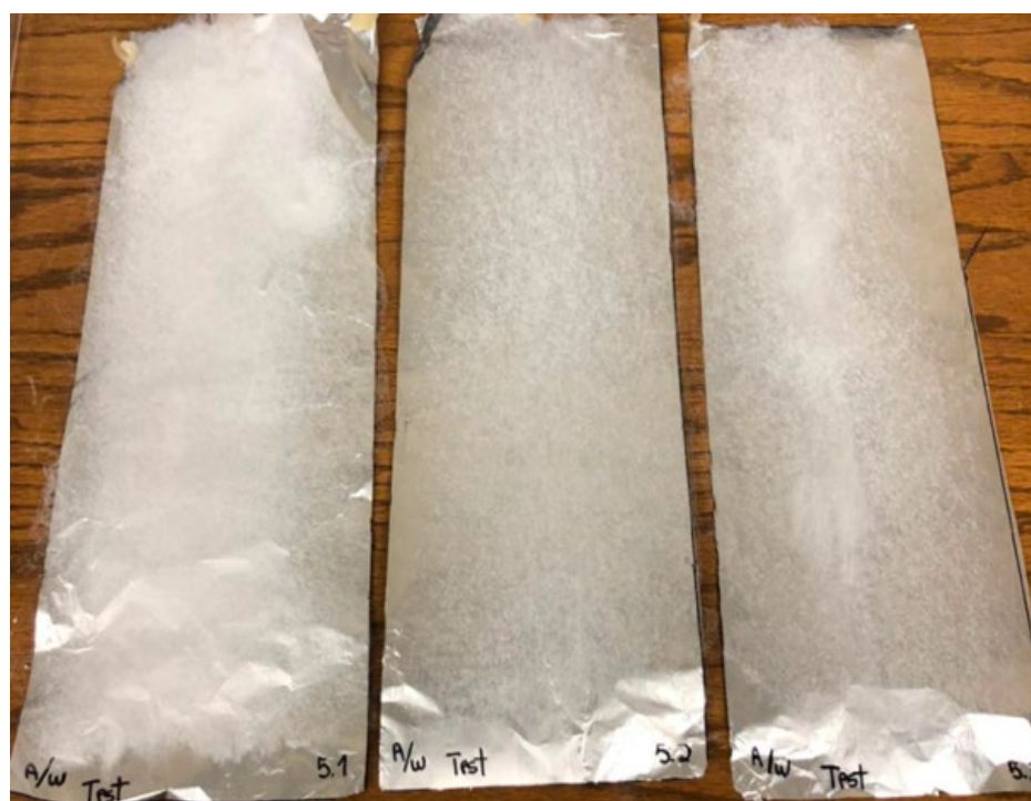
Figure 4.5 Photographic views of CNFs produced using solution 5 and rotating electrospinning technique
