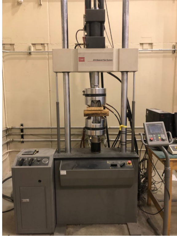
Figure 3.12 MTS ® 810 loading frame used to conduct the TSR test
