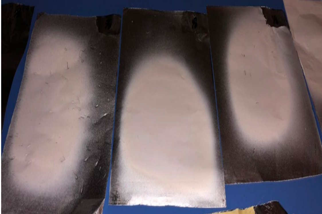
Figure 4.8 Photographic views of CNFs produced using solution 3 and static electrospinning technique
