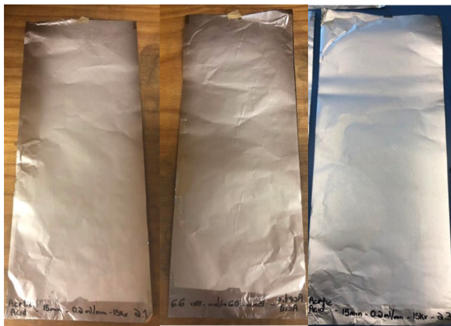
Figure 4.2 Photographic views of CNFs produced using solution 2 and rotating electrospinning technique
