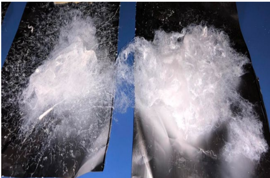
Figure 4.10 Photographic views of CNFs produced using solution 5 and static electrospinning technique
