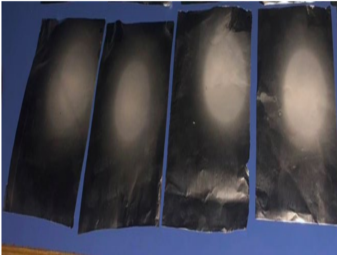
Figure 4.7 Photographic views of CNFs produced using solution 2 and static electrospinning technique
