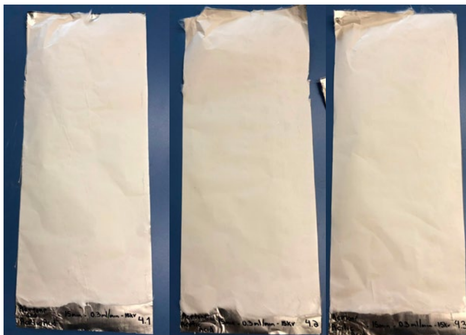
Figure 4.4 Photographic views of CNFs produced using solution 4 and rotating electrospinning technique
