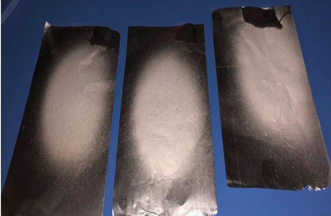
Figure 4.6 Photographic views of CNFs produced using solution 1 and static electrospinning technique
