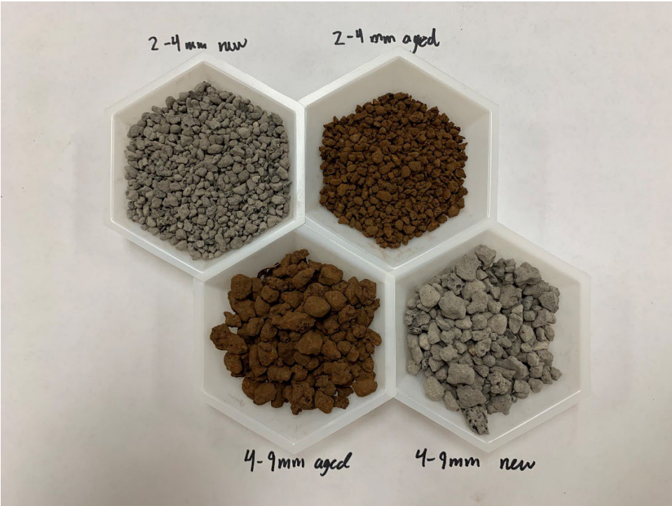
Figure 2.1 New and aged steel slag materials (top: 2-4 mm new, 2-4 mm aged; bottom: 4-9 mm aged, 4-9 mm new)
