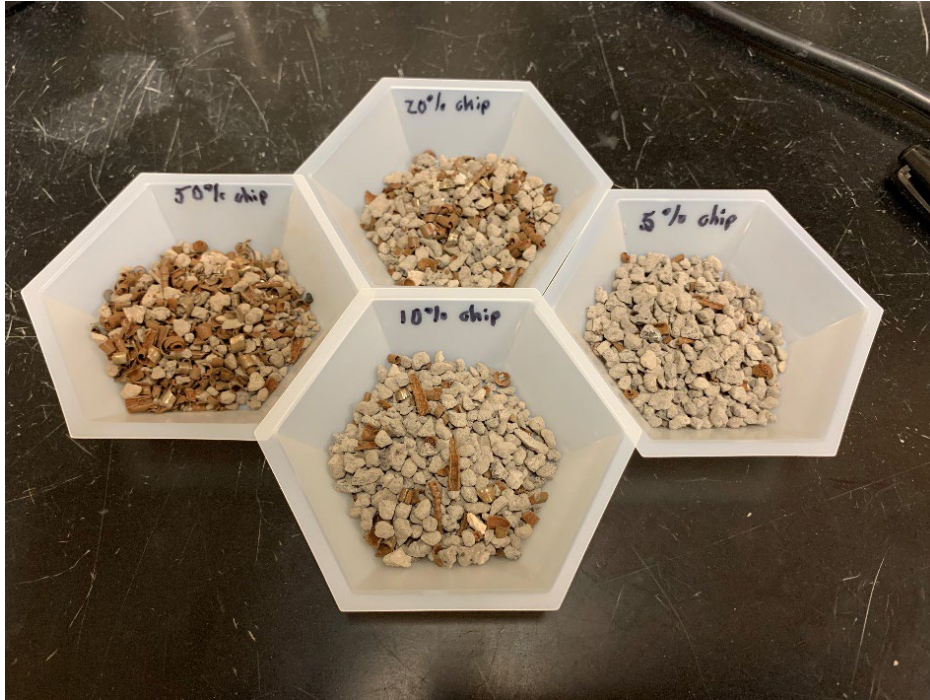
Figure 3.6 The mixed materials prior to being placed in the columns
