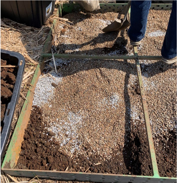
Figure 2.9 Adjustment of steel byproduct ratio in field filter
