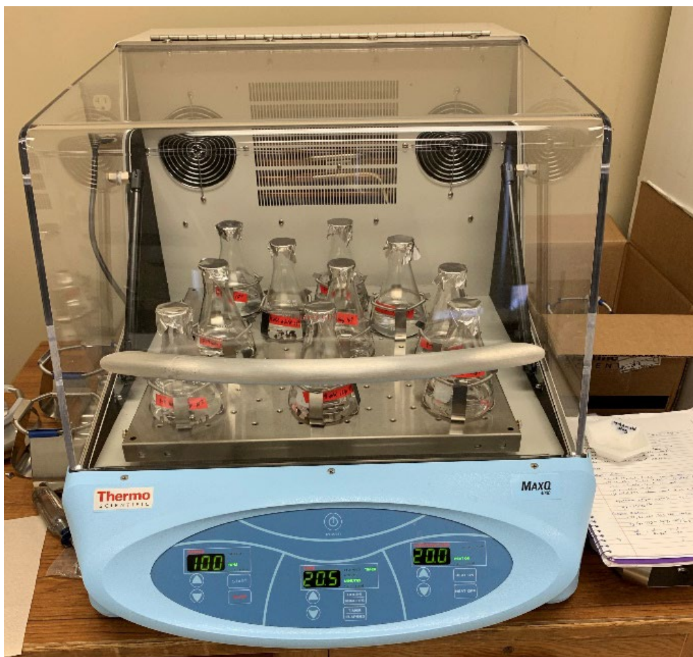
Figure 2.3 Benchtop orbital shaker used for batch studies
