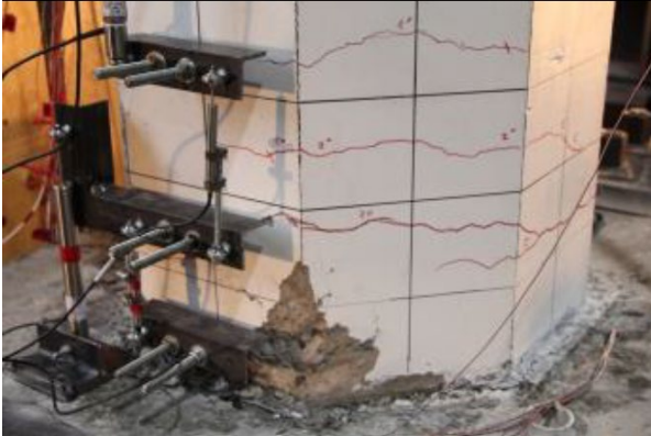
(a) Drift ratio=3% (cracks and spalling)
