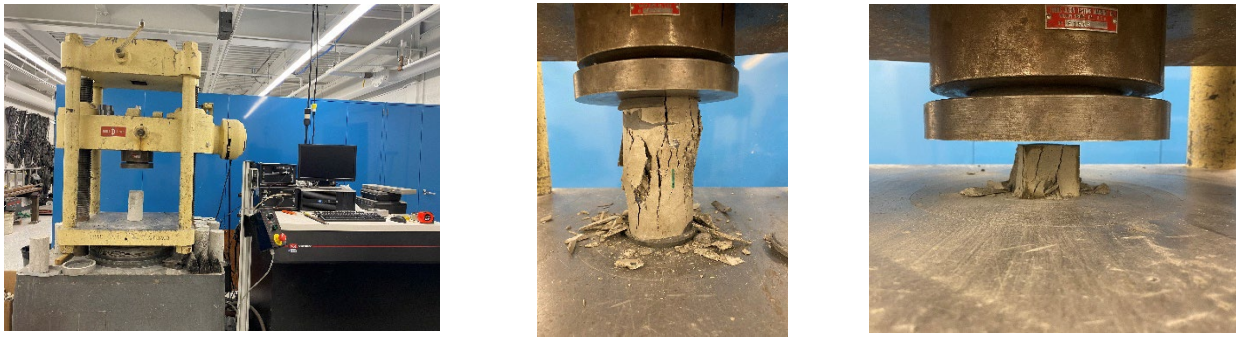
(a) Tinius Olsen compression machine (b) 4 in. × 8 in. cylinder (c) 2-in. cube
