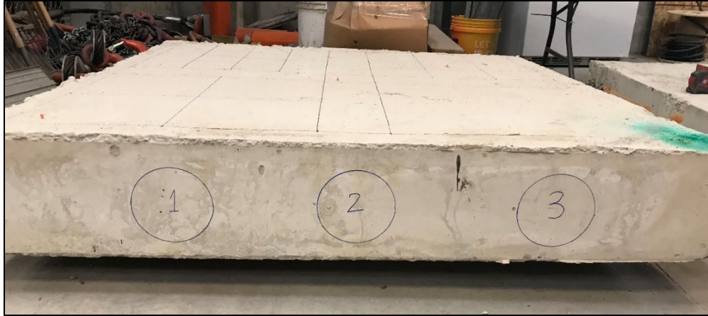
Figure 4.6 Circles located on the concrete side where the rebound hammer test is taken
