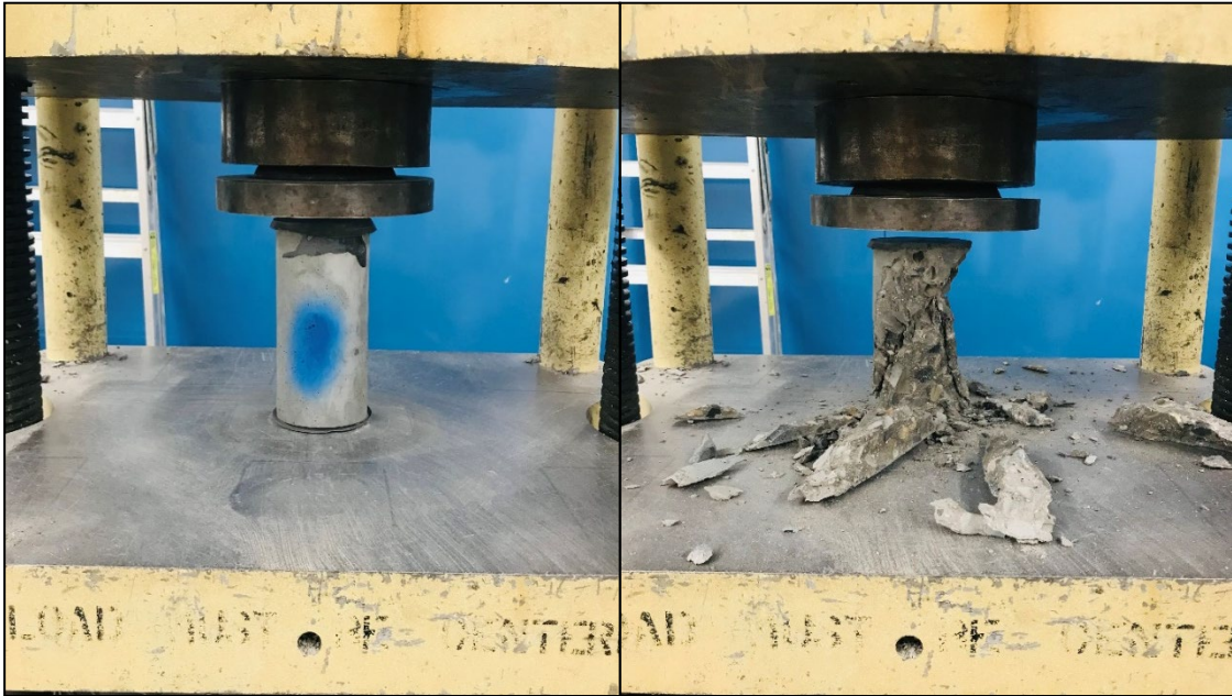
Figure 5.7 Compressive strength test, (a) before applying the loads, (b) after applying the loads
