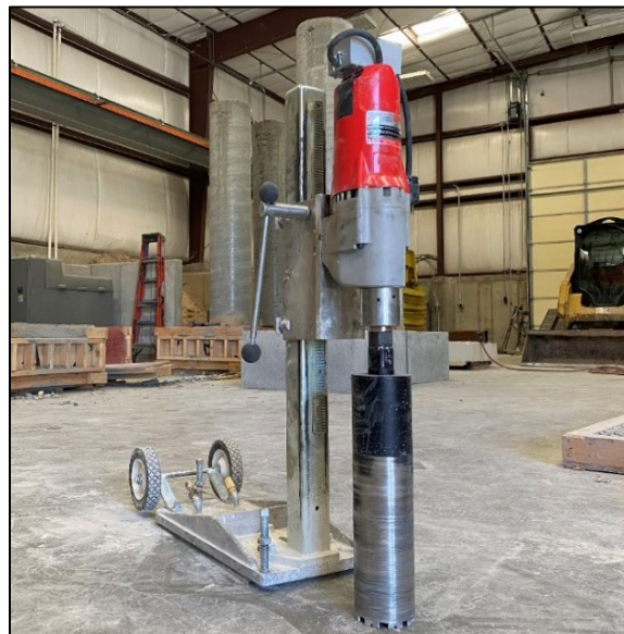
Figure 4.7 Concrete core test equipment
