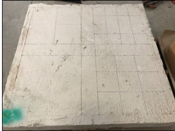
Figure 4.8 Preparation of the concrete slab before saw-cutting
