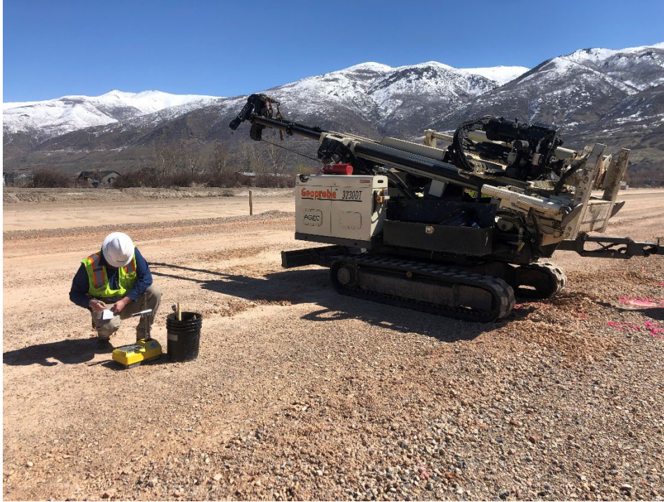
Figure 3.21 Nuclear density testing being performed and Geoprobe 3230DT onsite to perform CPT soundings
