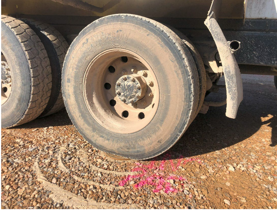
Figure 4.20 Photo of truck set of middle dual-passenger wheels centered over loading plate during TLT #1
