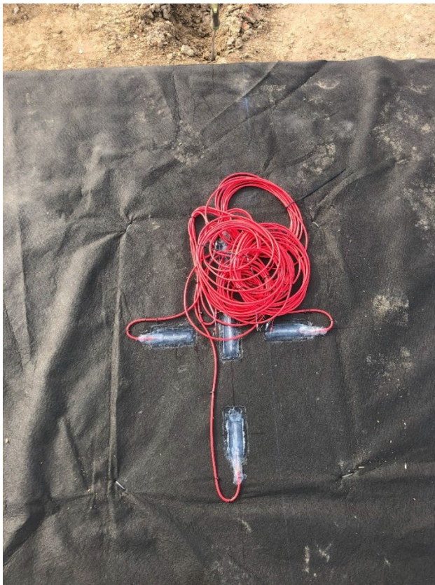
Figure 3.12 Geotextile with strain gages installed in the field
