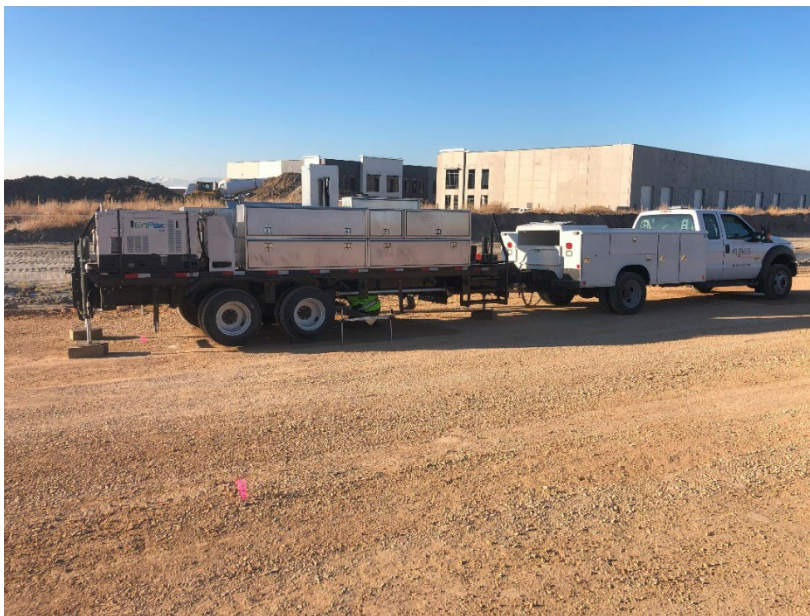
Figure 3.22 Ingios trailer mounted mobile APLT system
