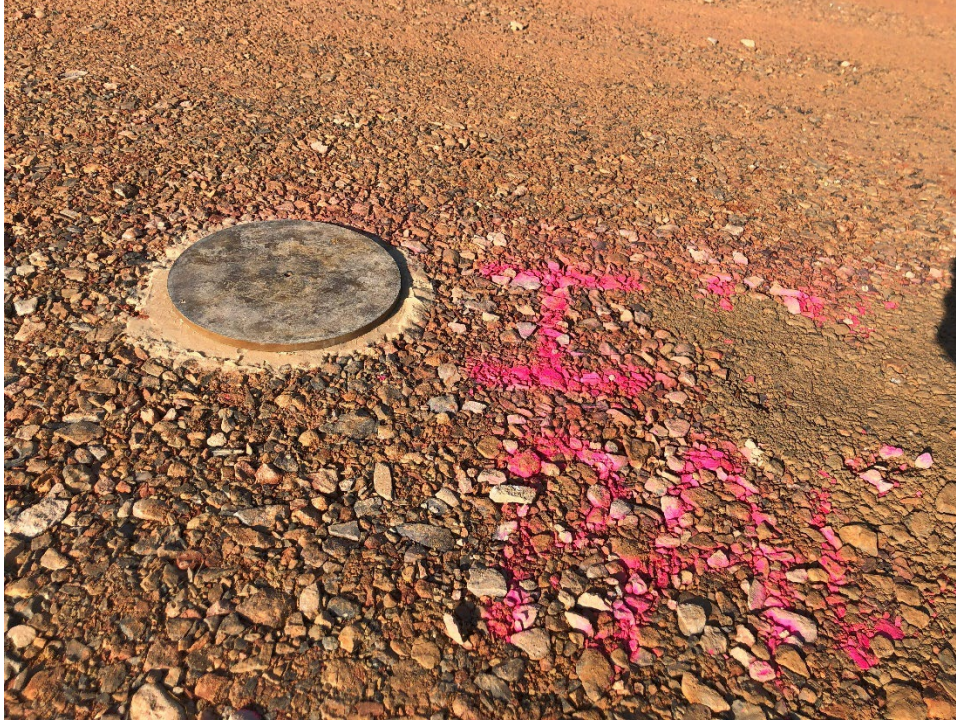
Figure 4.18 Steel loading plate used in TLT #1
