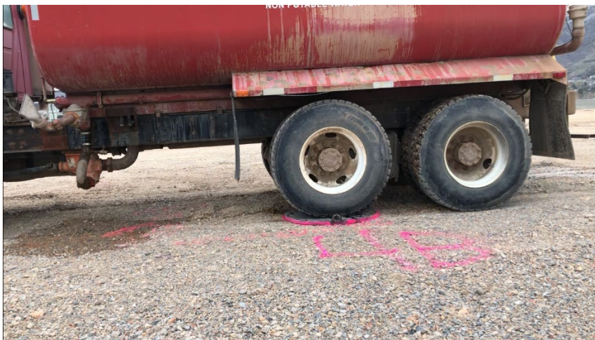
Figure 4.25 Water truck with driver-side set of dual wheels on the middle axle centered on the 34-inch diameter steel loading plate during TLT #2 at 4B
