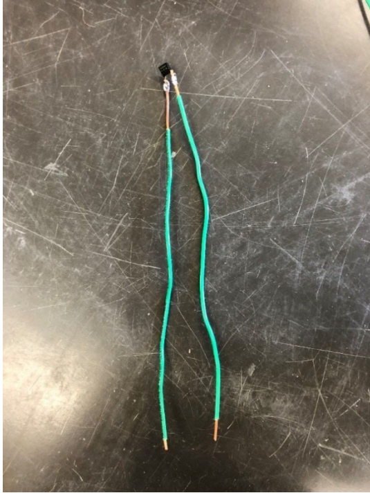
Figure 3.27 A precision resistor used for shunt calibrations
