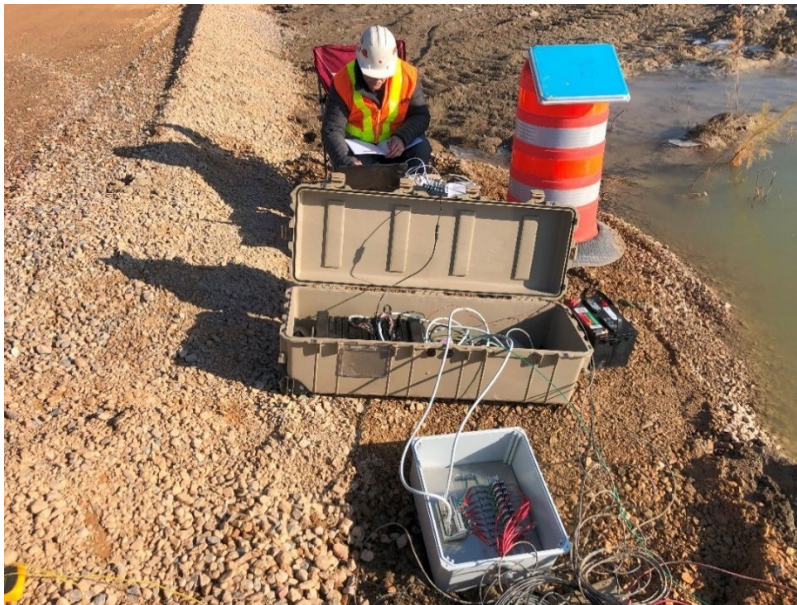
Figure 3.26 Photograph showing the CR9000x connected to a control box to collect strain gage data during an APLT test
