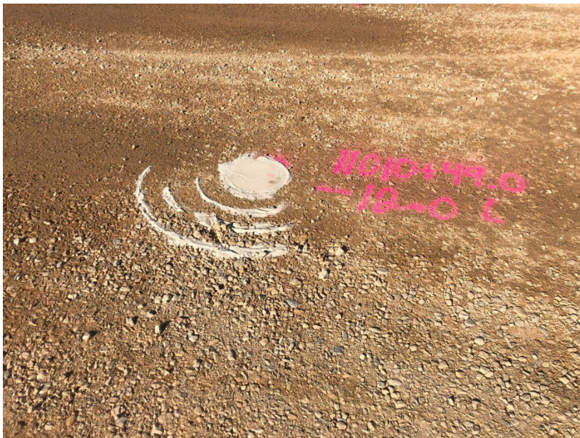
Figure 3.24 Sand used to ensure contact with the UTBC at the location of APLT after completion
