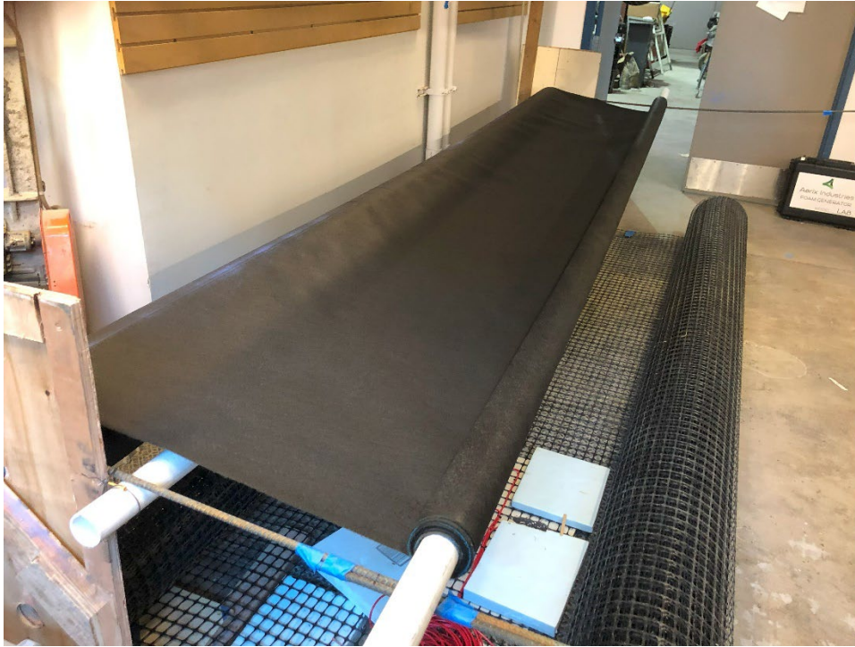
Figure 3.7 GT-180 and BX1200 geotextile and geogrid
