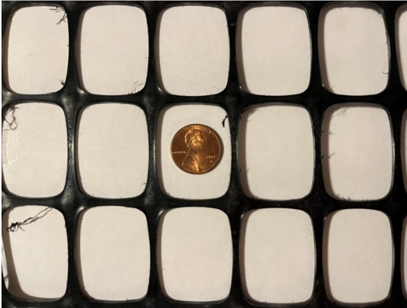
Figure 2.1 Up-close photograph of punched and drawn biaxial geogrid
