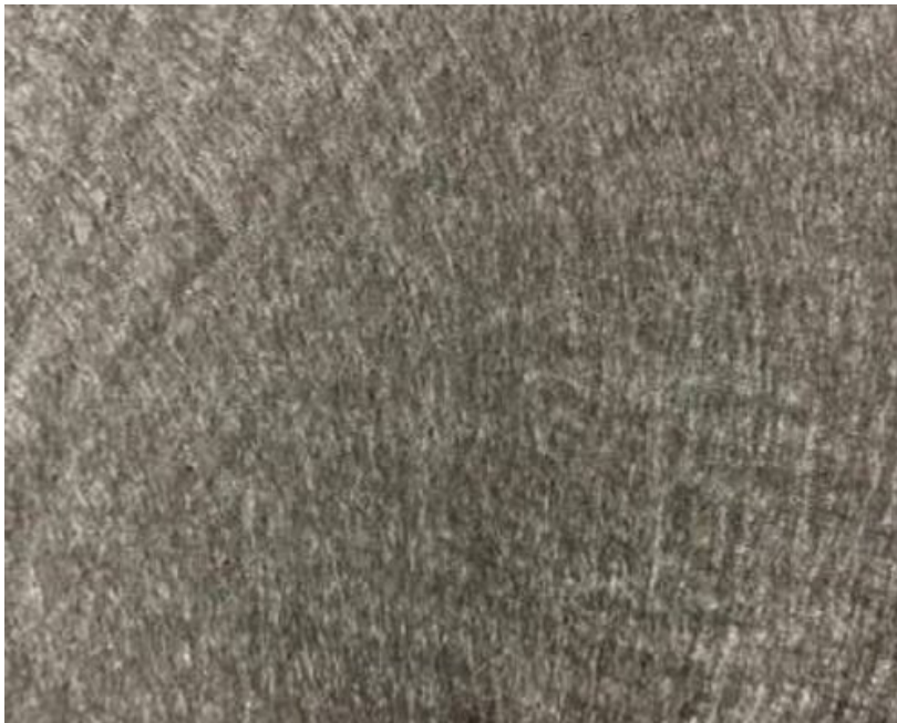
Figure 2.2 Up-close photograph of nonwoven geotextile
