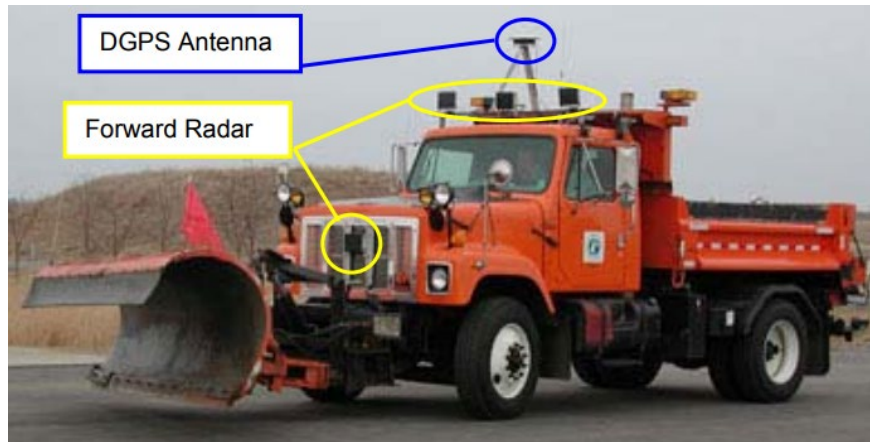
Figure E.3 Snowplow equipped with driver assistive system (DAS) technologies at MnROAD (25)
