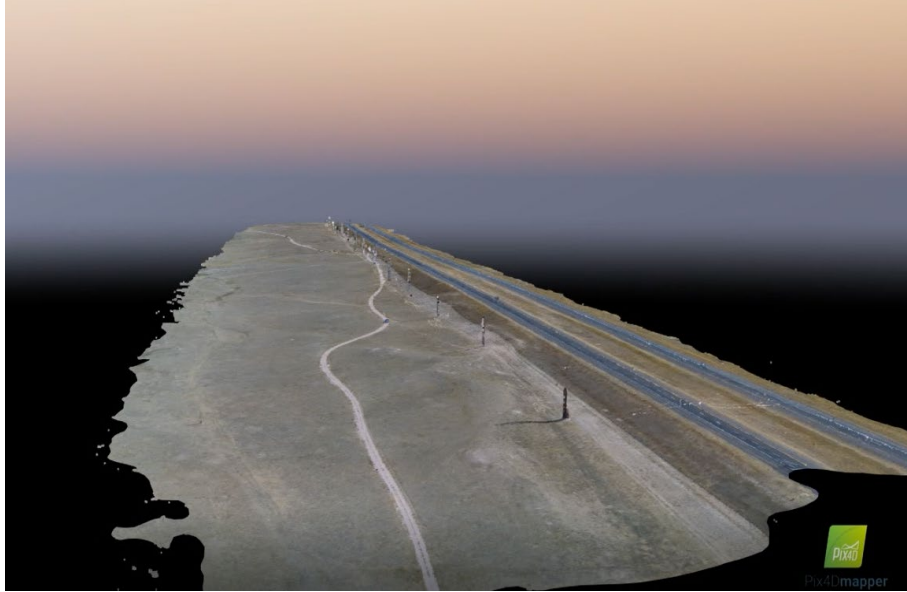
Figure 3.16 The 3D digital map created on PIX4D software of the proposed test track location in Zone 4
