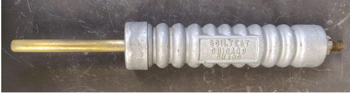
Figure 3.7 Harvard Miniature Tamper
