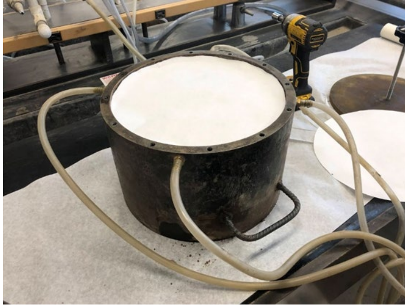
Figure 5.12 Filter Paper Placed in Bottom of LSC with Brass Fittings and Hoses Attached
