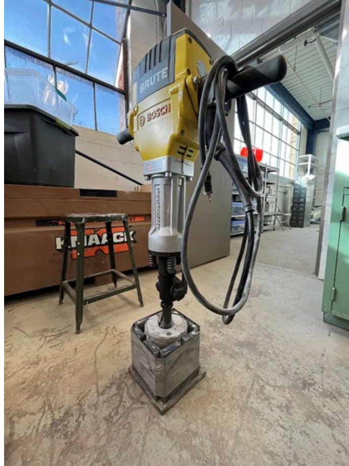
Figure 5.15 Electric Jack Hammer with Weights Attached to Square Compaction Plate
