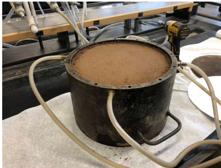
Figure 5.17 Bottom Plate and Top Plate Removed from LSC Containing Compacted Cohesive Material
