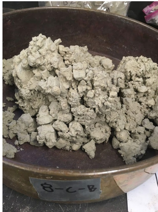
Figure 6.1 Photograph of a Sample of Untreated Base Course Material from SR-10 Near Emery, Utah
