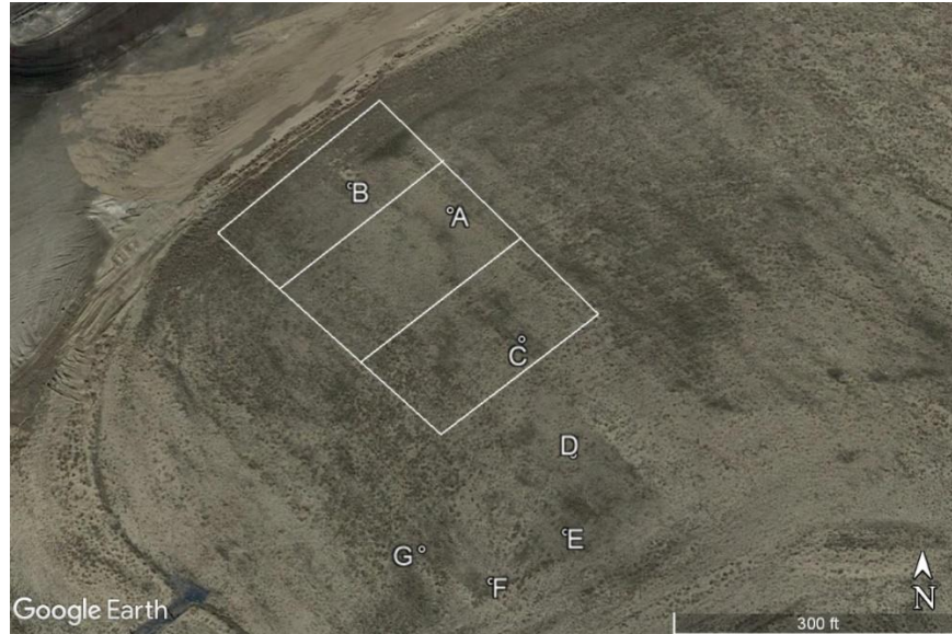
Figure 2.9 Sampling plan of fly ash in area 1
