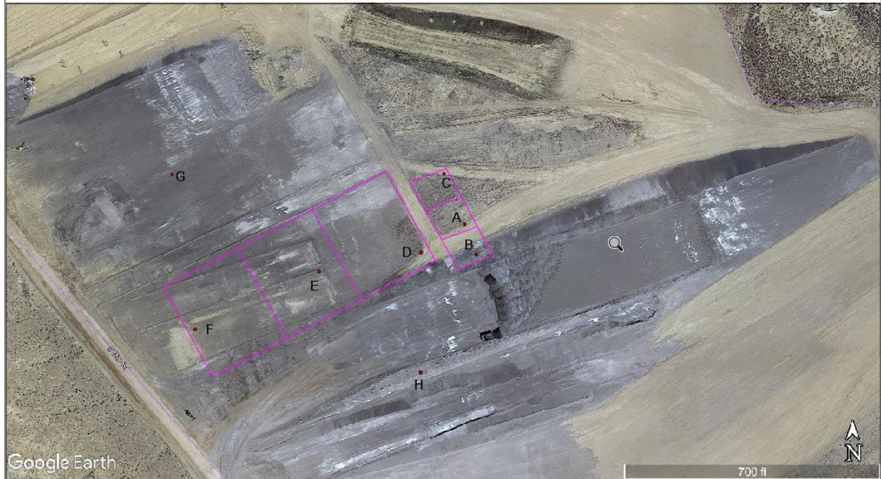
Figure 2.7 Sampling plan of fly ash in Jim Bridger Power Plant
