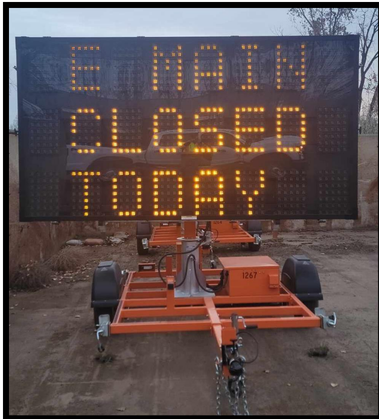
Figure 8 DMS (Public Work Department)
