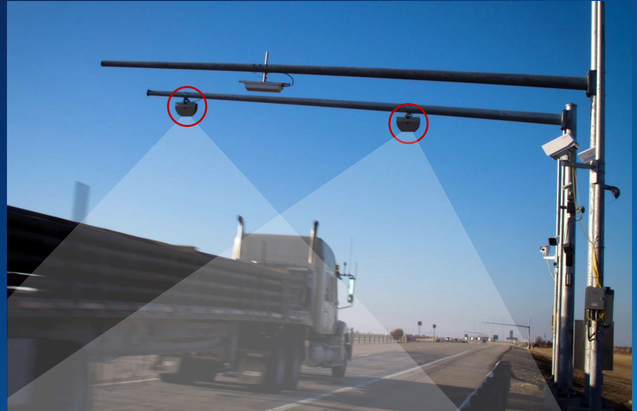
LiDAR Sensor Vehicle Dimensioning
