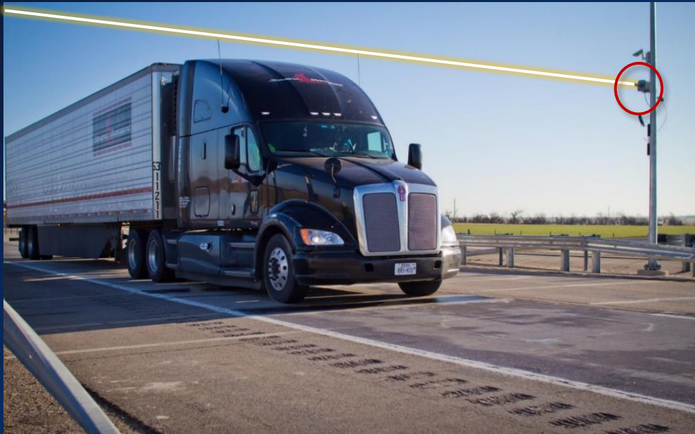
Red/Infrared Beam Overheight Detection
