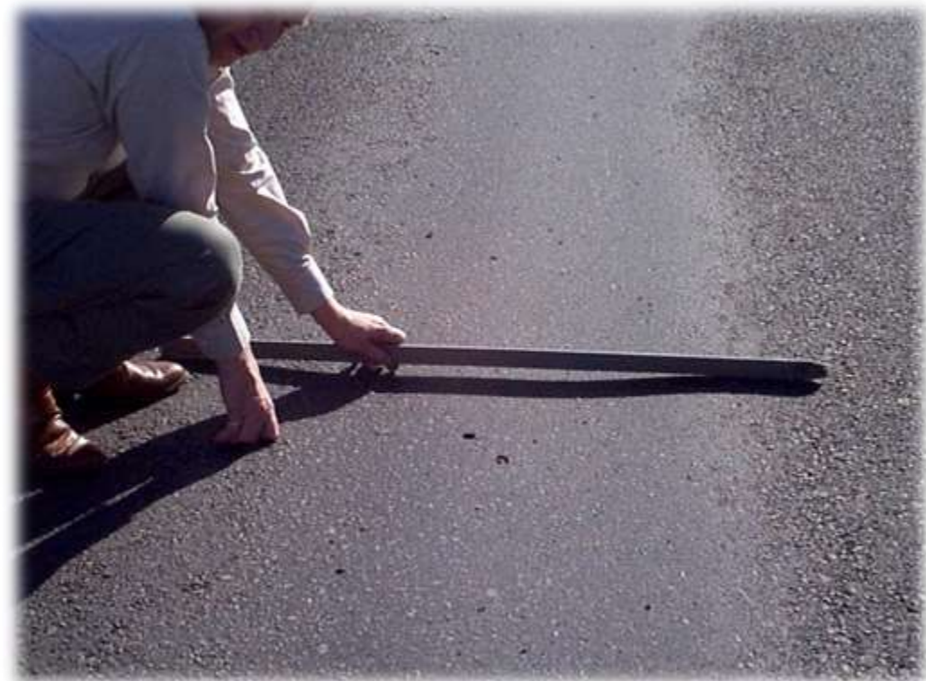
PG 67-22 unmodified, 15mm rut
