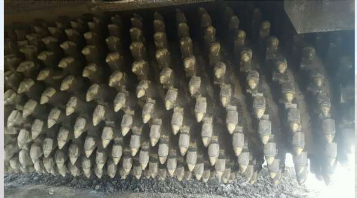
Micro milling head – more than 3x the number of teeth
