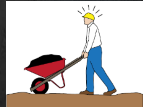
It takes much more effort to push the wheelbarrow through loose soil— in essence, MDP measures this effort by the soil compactor. The more compact the ground, the less energy is required to propel.
