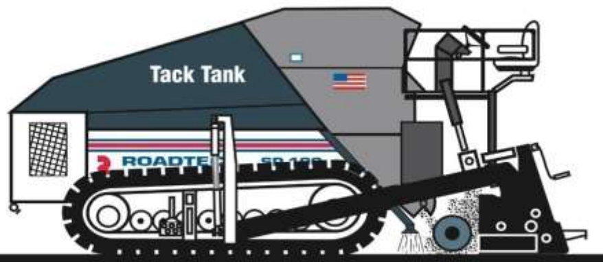
ROADTEC STEALTH PAVER WITH TACK TANK
