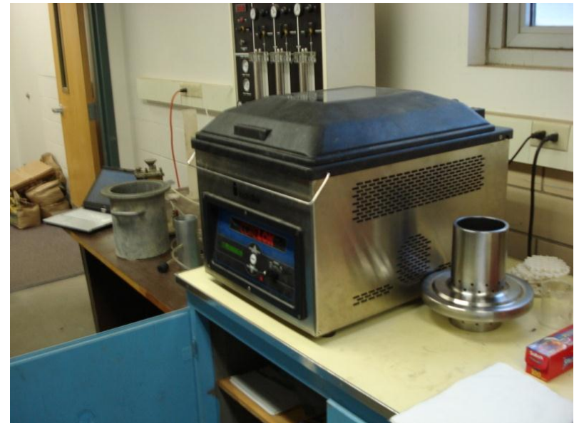
CoreLok for specific gravity determination.
