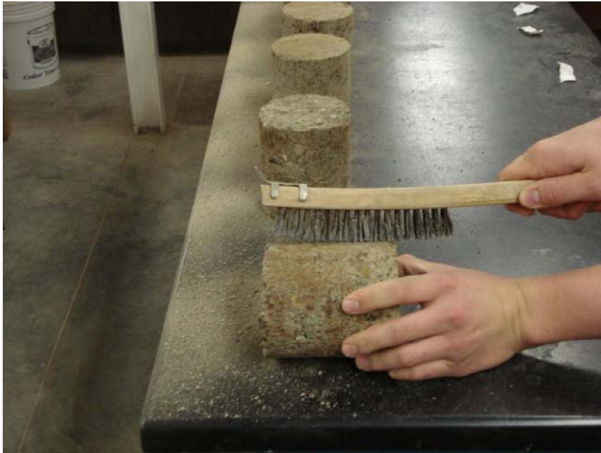
Moisture Sensitivity Testing with Wire Brush Method
